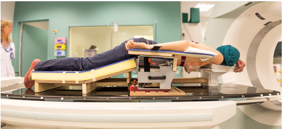
Fig. 8.9 Prototype iteration 2.3 with: thin fibreglass upper shell, indexed sheet metal hip module, adjustable fibreglass arm support, elevated leg support with slight flex in hip- and knees for improved comfort, flat head support region for different head modules.
