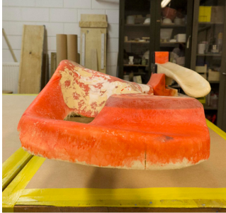
Fig. 7.7 Front view of iteration BBV6, laminated with fibreglass and polyester resin for added strength.
