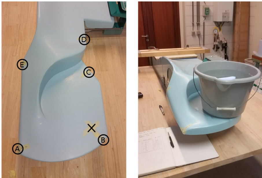
Fig. 10.3 Load testing of intern frame. A load of 100N was applied at point X.
