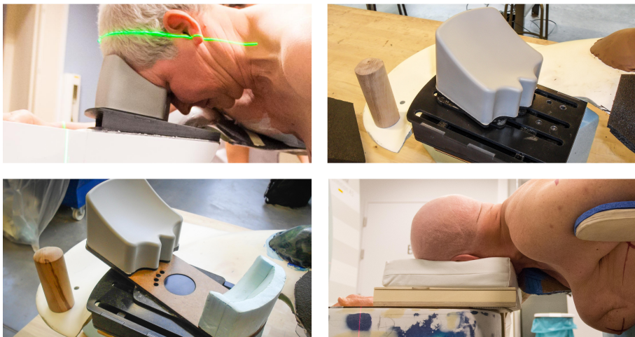
Fig. 8.4 4 different head support prototypes: top-left: H_1, H_2, H_4 ; top-right: H_1, H_2, H_4, H_5 ; bottom-left: H_1, H_2, H_3, H_4, H_5 ; bottom-right: H_6 .
