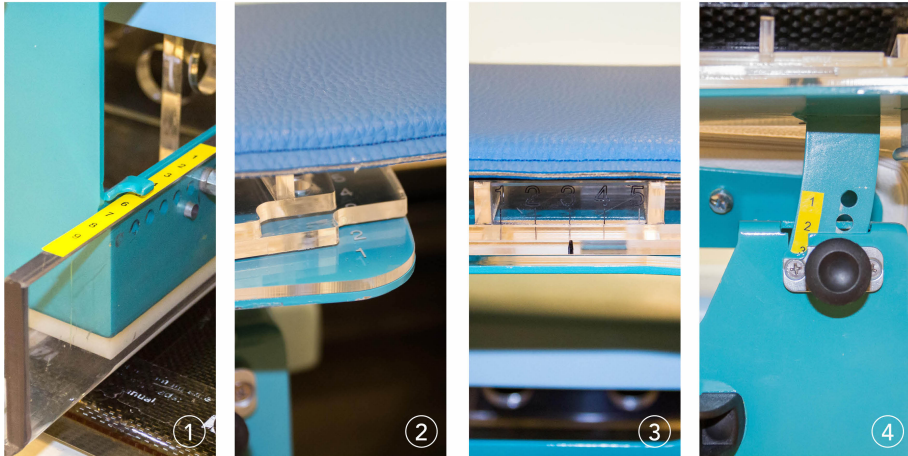
Fig. 9.4 Sheet metal arm module with indexed positioning: 1) latero-lateral adjustment for arm module on baseplate; 2) arm support blade resting on the arm module baseplate; 3) craniocaudal adjustment of arm support blade; 4) pitch adjustment.
