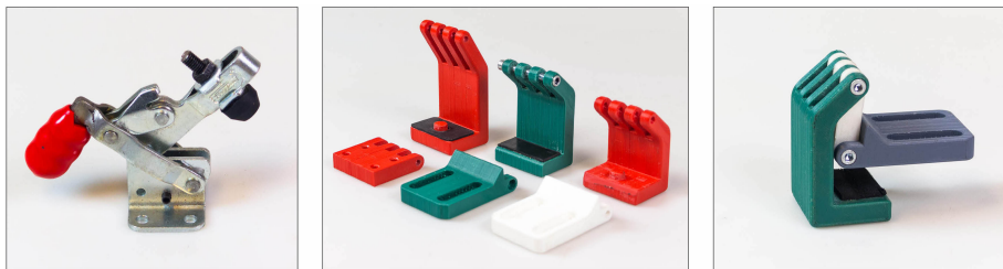
Fig. 9.8 Different fixation prototypes for BC2. Left: modified clamp, Middle: Exploration of different clamping systems, Right: Final assembled clamping system.
