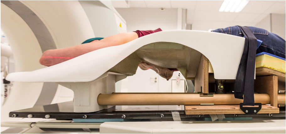
Fig. 8.8 New breast board with aramid honeycomb core, positioned on the CT-simulation table. The thin shell structure results in enlarged beam access range.
