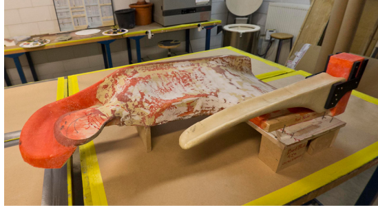
Fig. 7.8 Iteration BBV6 with the new gutter shaped contralateral arm support and the wedge's concave contralateral breast region.
