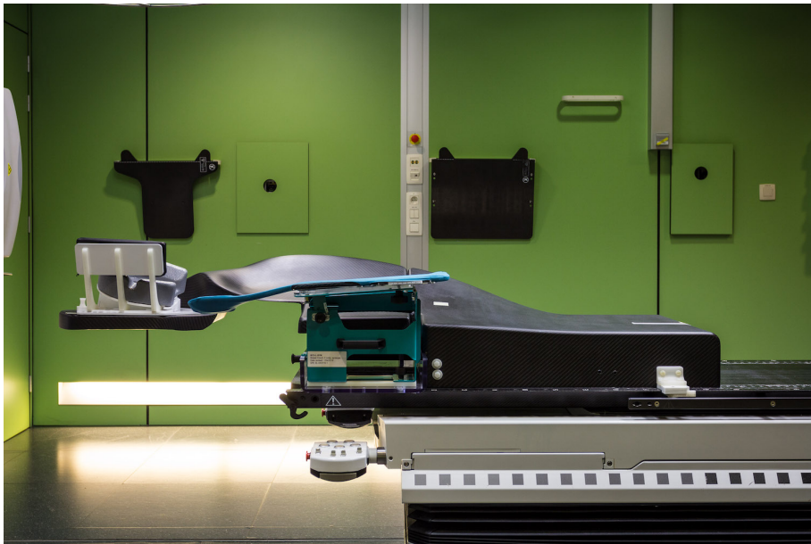
Fig. I.5 Final breast couch iteration BC3-L, positioned on the LINAC table.
