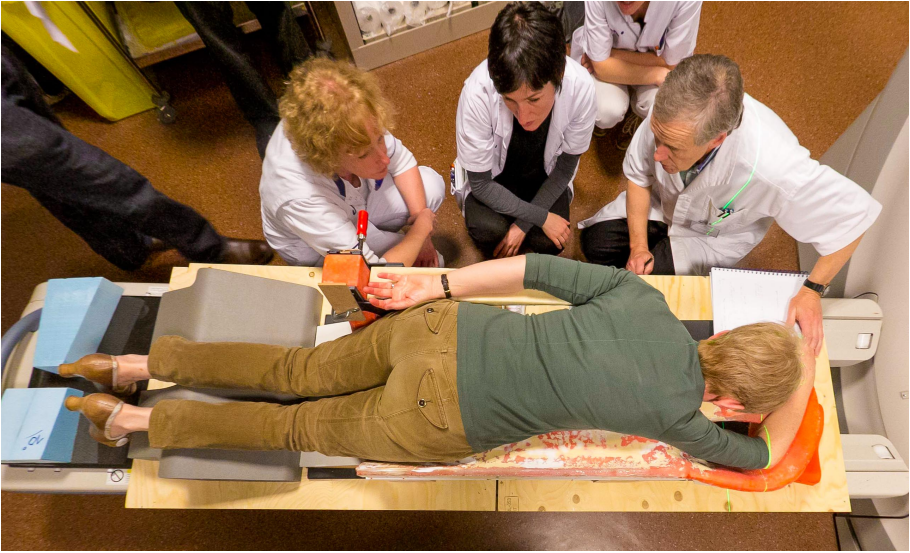
Fig. 3.2 Example of a small user test during an early prototype iteration (Phase I). Several team members (nurse, patient, physician, physicist and designer) are testing, evaluating and modifying new patient positions.
